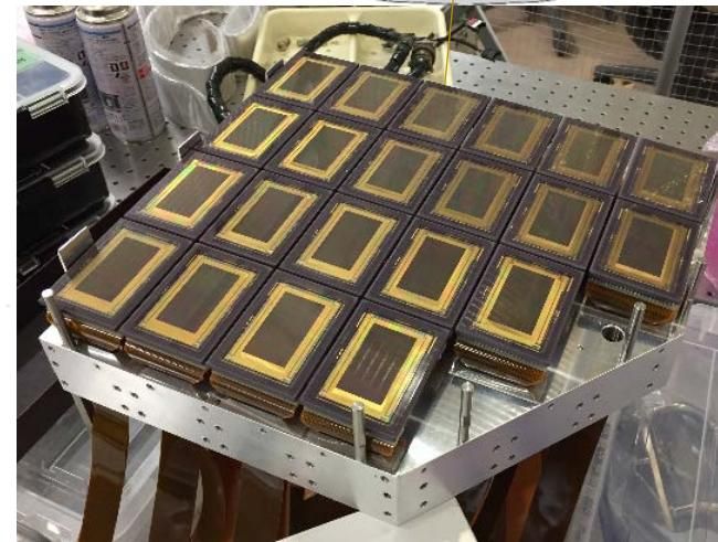
21 chips of CMOS sensors of Q1
