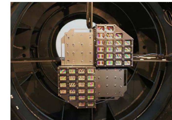
Q1 and Q3 cameras on Schmidt telescope
