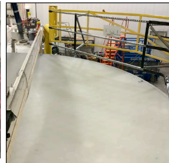
TAO 6.5-m mirror with front surface generated with 100 mesh metal bond cup wheel.
