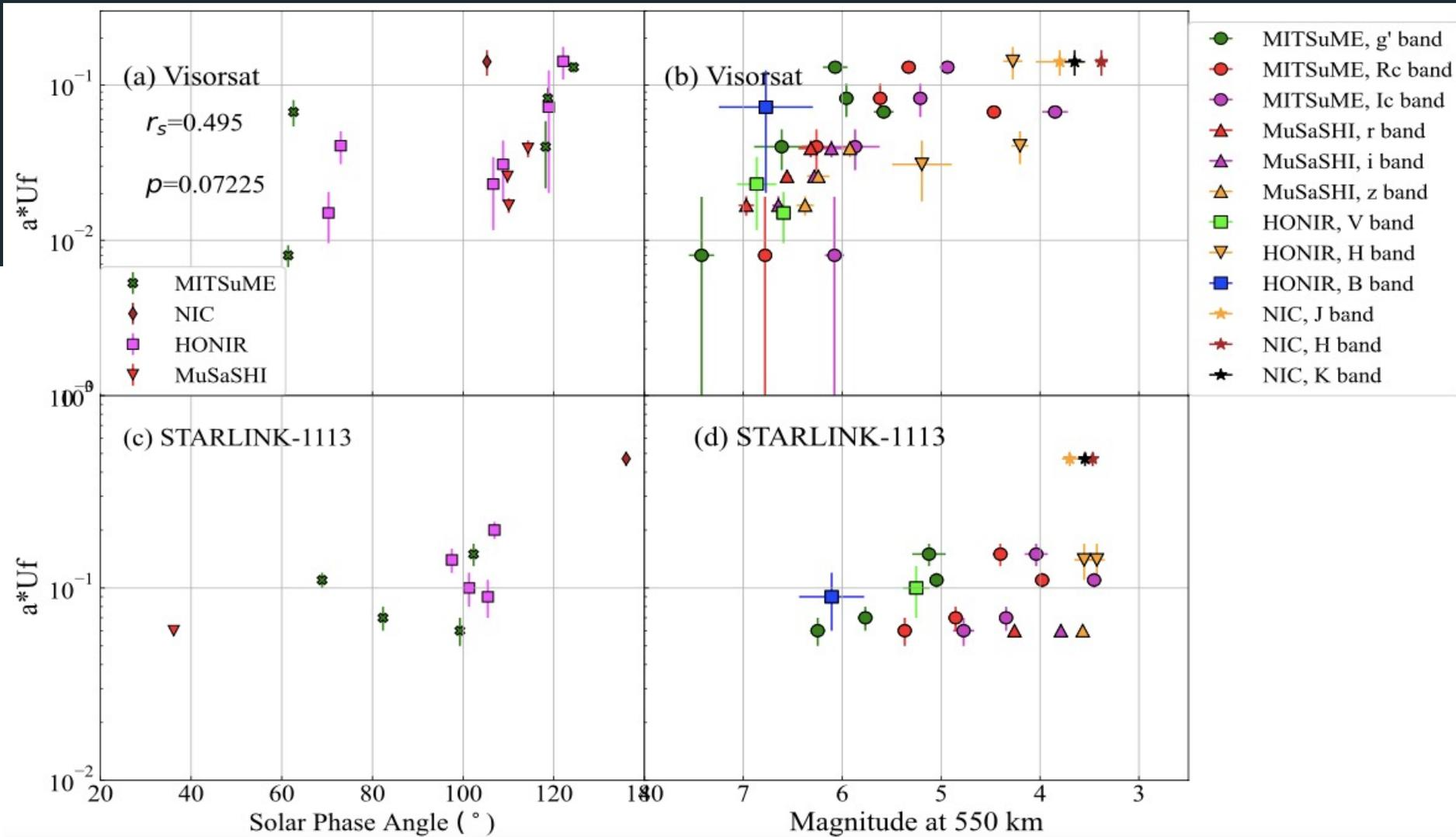
The smaller the covering factor is, the brighter the magnitudes of Visorsat tend to become.
